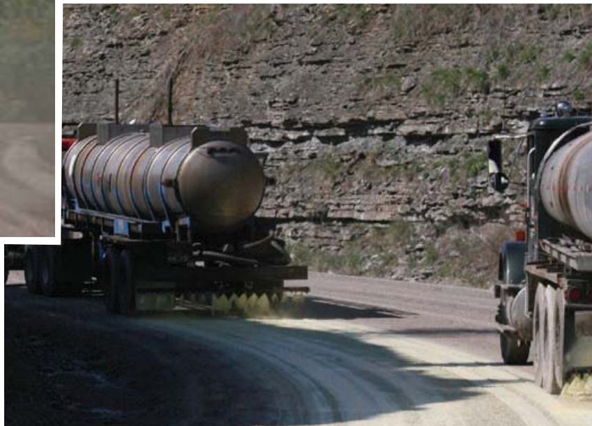
Haul road is spray treated to prevent coal dust.
