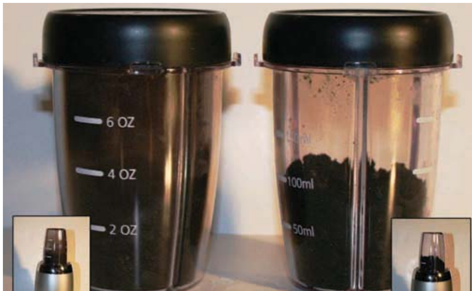
Untreated and treated coal after “mixing” in a high speed blending. No dust is generated in this test when treated with AKJ DC-2008.
